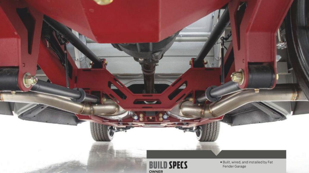
would put this C10 build undoubtedly straight to the top of anyone's "best of" list. The foundation: a full bumper-to-bumper frame from Porterbuilt Fab. But this wouldn't be just a standard LS Powered/Porterbuilt combo rolling on 22s. Tony decided that the rolling chassis would be the foundation and direction for where this "super-truck" build would head. A 2018 Chevy Performance 6.2L direct-injected LT4 supercharged V-8 mated
